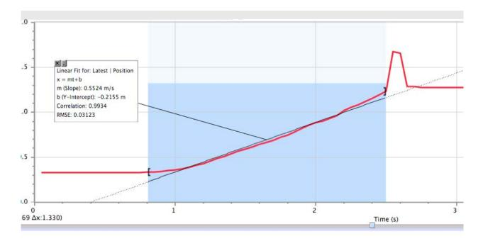
Use the computer and sensors to measure gravity by inclining the track by a small amount (the feet of the track can be unscrewed to raise the track) and measuring the cart's average velocity and acceleration. Again, compare your observations to your predictions.
